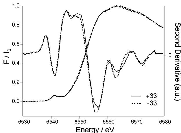
FIGURE 7: Normalized Mn K-edge XANES spectra and their second derivatives of untreated (solid trace) and 33 kDa protein-depleted (dotted trace) PS II membranes. Each trace is the average of the spectra from three independent PS II preparations.
