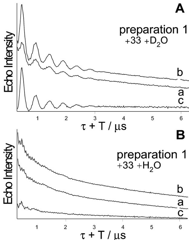
FIGURE 3: Time-domain three-pulse ESEEM traces of undepleted PS II membranes from preparation 1 equilibrated with D<sub>2</sub>O (panel A) or H<sub>2</sub>O (panel B) buffer in the S<sub>1</sub> (traces a) and S<sub>2</sub> (traces b) states. The difference traces (traces c) are trace b minus trace a, respectively. The traces have been offset for clarity. For instrumental parameters, see Figure 4.
