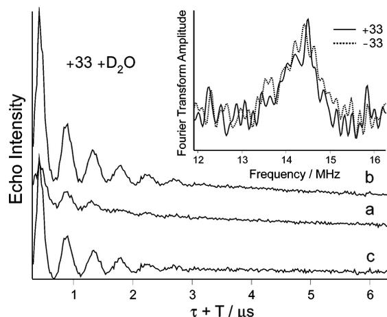
FIGURE 5: Time-domain three-pulse ESEEM traces of undepleted PS II membranes in  $D_2O$  buffer from preparation 3. Traces a–c and instrumental parameters are as in Figure 4, except a  $\tau$  value of 238 ns was chosen to maximize  $^1H$  modulation. Inset: Fourier transform spectra of the normalized difference traces (c) of the undepleted (solid trace) and 33 kDa protein-depleted (dotted trace) samples, showing the region around the proton Larmor frequency.
