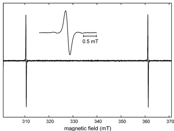
**Fig. 2.** Experimental X-band spectrum of H@iBuT<sub>8</sub>, acquired at 9.4801 GHz and 292 K with 0.1 mT modulation amplitude. Inset: enlarged low-field line.
