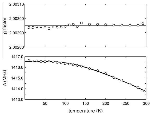
**Fig. 3.** Temperature dependence of the  $g$  factor and the hyperfine coupling of H@iBuT<sub>8</sub>, measured at 9.48 GHz and 1  $\mu$ W. Dots: Experimental values with errors  $\pm 0.00006$  for  $g$  and  $\pm 0.2$  MHz for  $A$ . Lines: average of  $g$  values (2.00294), fit of three-dimensional oscillator model [39] to  $A$  values ( $c_0 = 0.00332$ ,  $c_2 = -0.89$  nm<sup>-2</sup>,  $k = 5.1$  N m<sup>-1</sup>).
