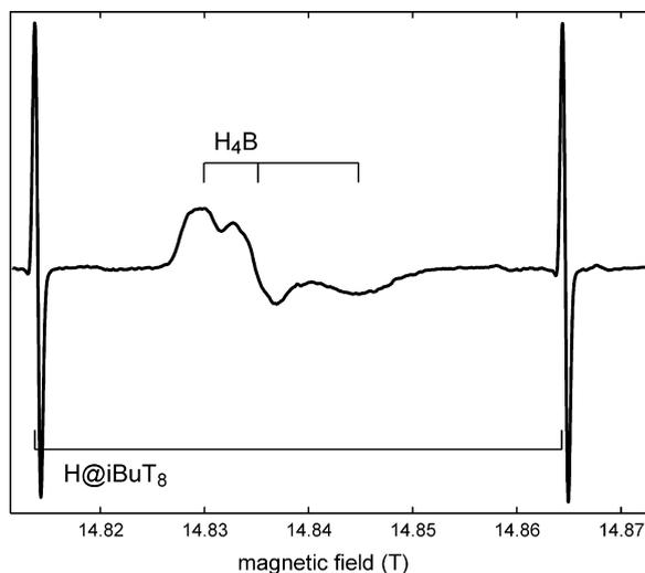
**Fig. 6.** cw EPR spectrum of the tetrahydrobiopterin ( $H_4B$ ) radical in the heme domain of inducible nitric oxide synthase (iNOS), measured at 416 GHz and 50 K, sweep rate 0.021 mT/s, modulation 1 mT at 50 kHz.
