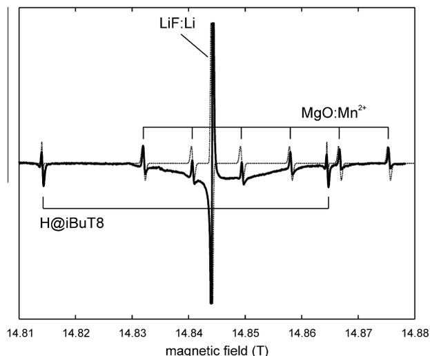
**Fig. 5.** 416.000 GHz spectra of H@iBuT<sub>8</sub>, together with LiF:Li and MgO:Mn<sup>2+</sup>, recorded at 60 K. Sweep rate 0.1 mT/s, modulation 0.1 mT at 50 kHz. Dashed line: simulation.
